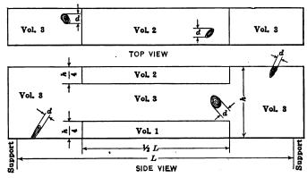
Fig. 31.—Division of beam into volumes for location of knots. Measurement of knots on horizontal and vertical face of beam. d = diameter of knot.
